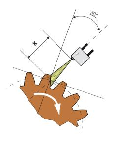
The number of nozzles varies depending on the length of the tooth flank. They are positioned at a distance X, generally  $200 \pm 50$  mm. Optimum lubrication is obtained when the spraying image covers the entire surface of the teeth.
